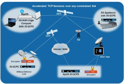
XipLink Operating System (XipOS) is a scalable and robust network operating system providing bridging and routing functionality to support flexible deployment scenarios. To increase overall effectiveness, XipOS provides a hierarchical class-based QoS mechanism enforcing minimum, maximum and shared bandwidth configurations for traffic shaping of multiple sites, users and applications/services.
