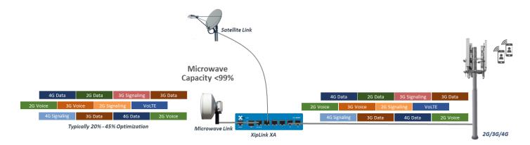
Figure 1. MBTS will optimize the backhaul link and keep all traffic on microwave if capacity is under 100%
