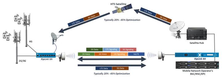
Figure 3. XipLink MBTS is configured to overflow the download data to satellite only. All upload traffic will stay on the microwave.
