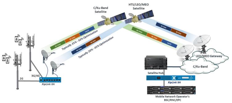
Figure 4. Using XipLink MBTS to carry voice and signaling traffic via highly reliable C-band satellite and sending data via best-effort Ka band satellite.
