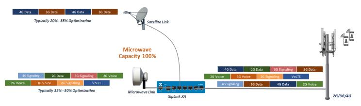
Figure 2. XipLink MBTS allows MNO to re-use existing microwave links for high-value voice and signaling traffic while using low-cost backhaul such as HTS satellite, MPLS, or DSL for data traffic.
