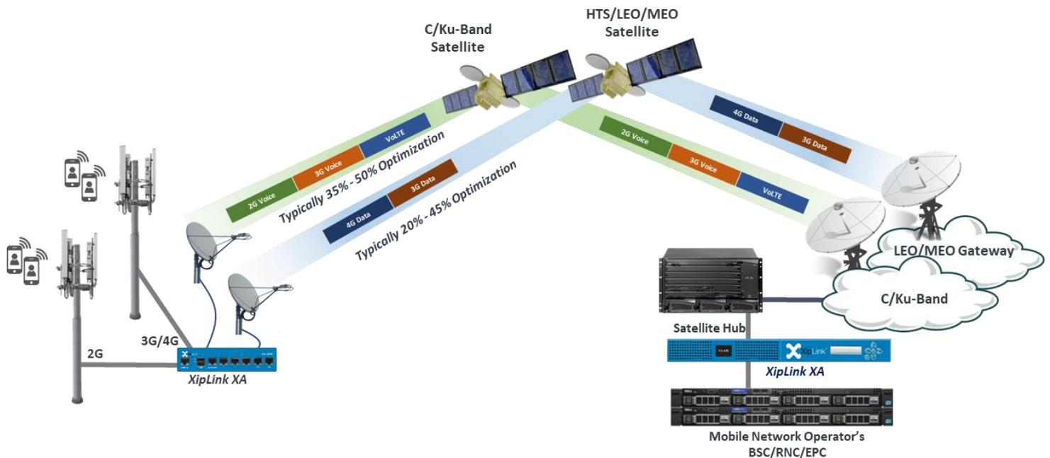
Figure 4. Using XipLink MBTS to carry voice and signaling traffic via highly reliable C-band satellite and sending data via best-effort Ka band satellite.
