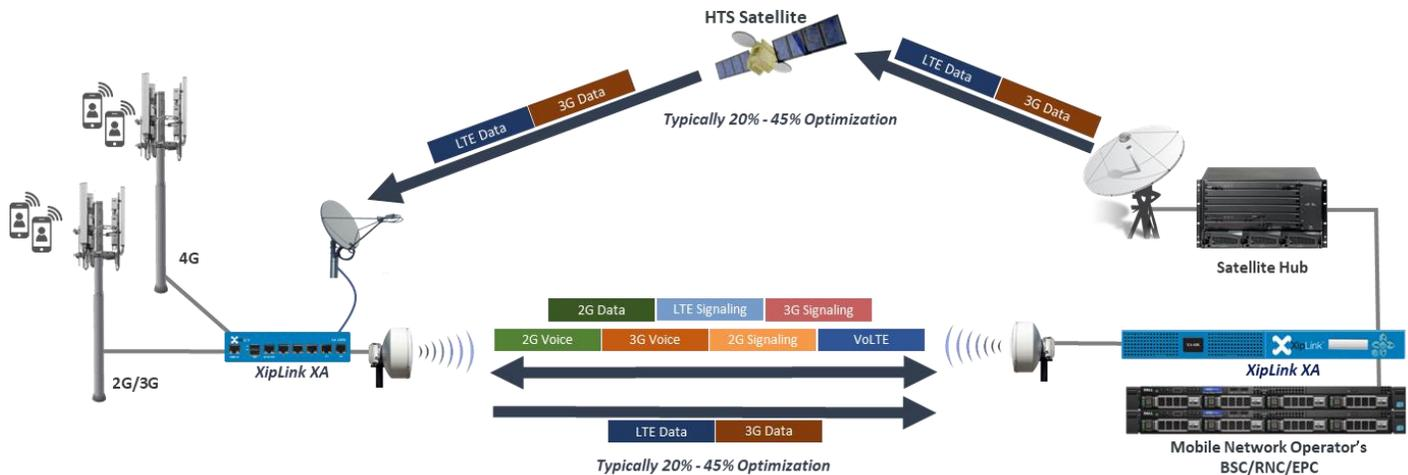
Figure 3. XipLink MBTS is configured to overflow the download data to satellite only. All upload traffic will stay on the microwave.
