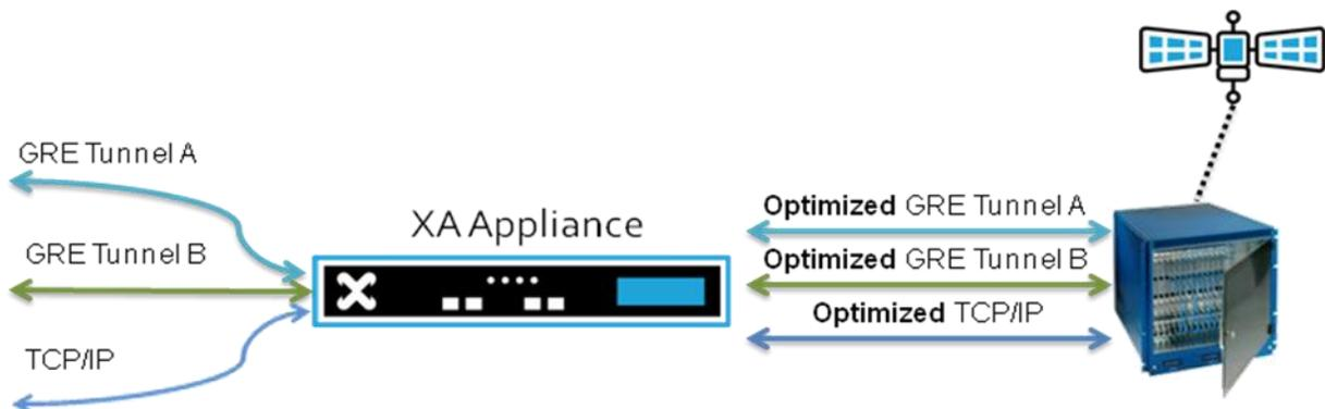
The feature is performed locally and requires no configuration or negotiation with other XA units. This enables topologies where the GRE tunnel may occur in a router after a remote XA performs the optimization, but then the optimized GRE encapsulated IP arrives together at another XA unit. An example topology is shown below.
